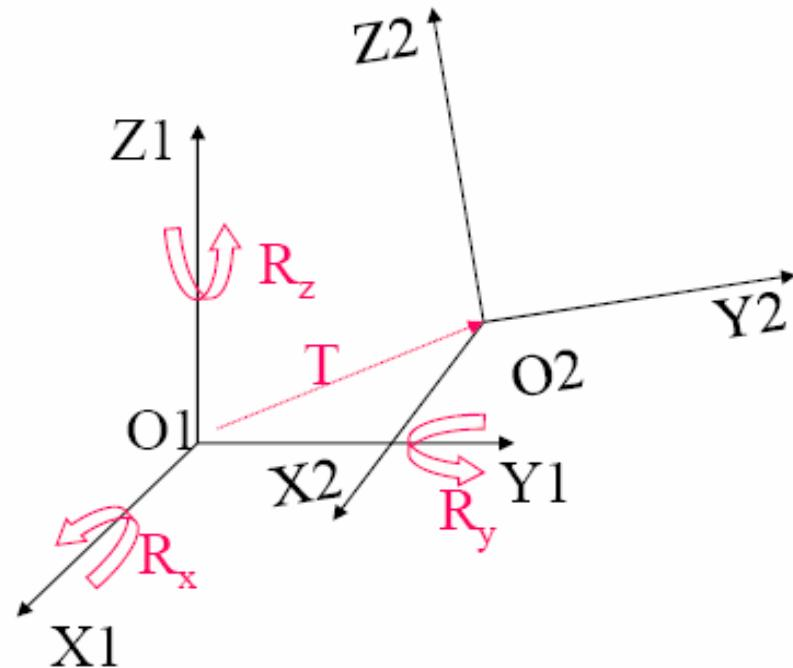
$$\begin{pmatrix} X \\ Y \\ Z \end{pmatrix}_2 = \begin{pmatrix} X \\ Y \\ Z \end{pmatrix}_1 + \begin{pmatrix} T_x \\ T_y \\ T_z \end{pmatrix} + \begin{pmatrix} D & -R_z & R_y \\ R_z & D & -R_x \\ -R_y & R_x & D \end{pmatrix} \begin{pmatrix} X \\ Y \\ Z \end{pmatrix}_1$$
